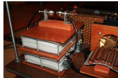
Figure 4.11: An unit of v.3 ; both units connected in series and mounted on Zeus' chassis.
