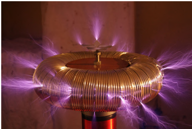
Figure 4.32: Numerous sparks arising from the top load asperities. Notice Zeus' Eagle. 1s shutter speed.
