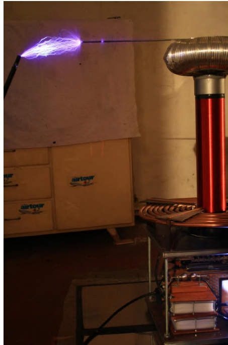
Figure 4.13: This capacitor has indeed driven Zeus, and eventually did not fail. 1s shutter speed.
